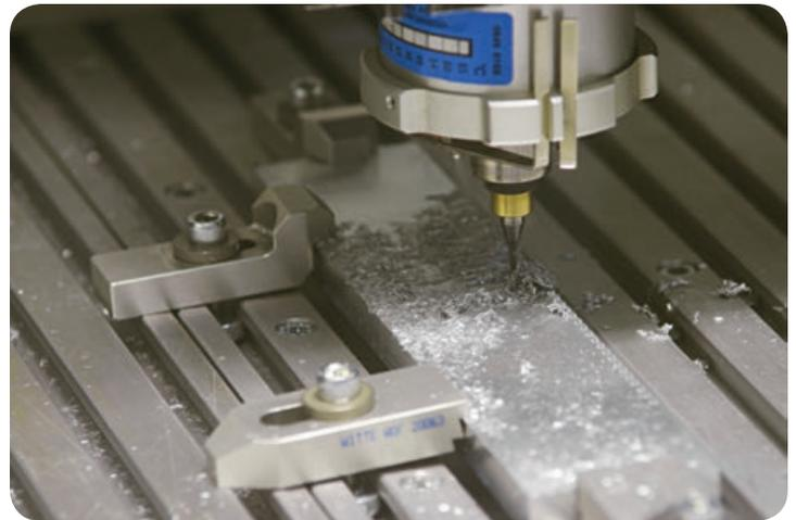
Reaming is difficult, and tool life is very low compared to that obtained in machining heat-treated, low-alloy steel.
